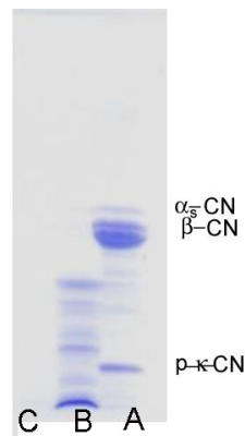
Figure 2. Sodium dodecyl sulfate–polyacrylamide gel electrophoresis (SDS-PAGE) of whole Sjenica sheep cheese before digestion (A), after pepsin digestion (B) and after pepsin + pancreatin digestion (C).
