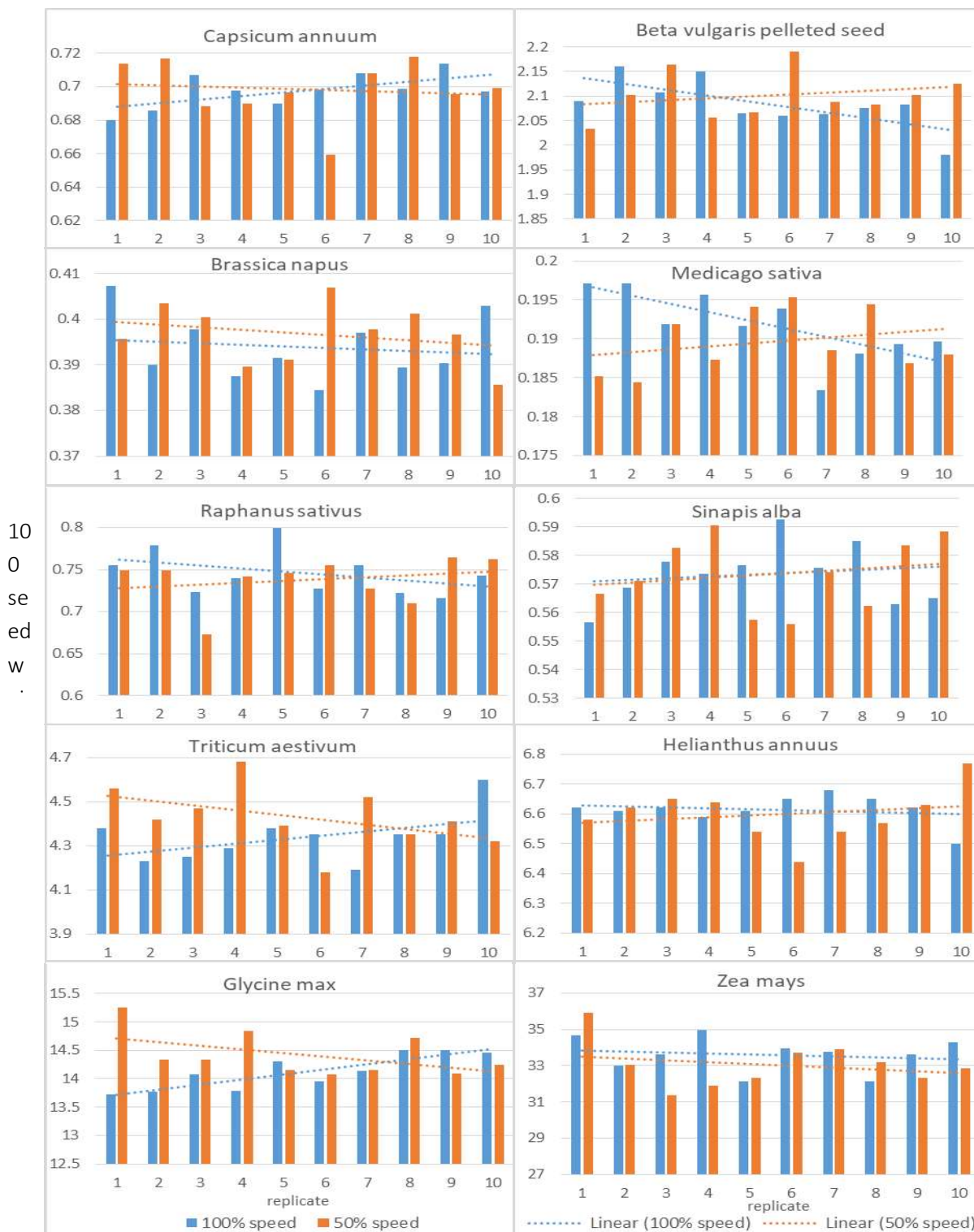
Figure 2. Hundred seed weight in 10 replicates for 10 species obtained by counter at maximum (blue bar) and reduced speed (orange bars) and related linear trend lines
