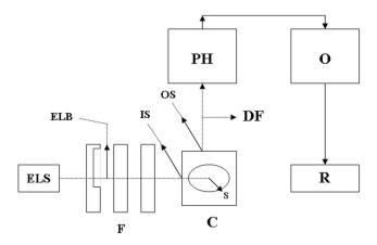
Figure 1. Experimental setup of the photosynthetic fluorescence method and the measuring equipment for delayed chlorophyll fluorescence: ELS - excitation light source; F filters; ELB - excitation light beam, IS - input dark chamber slot, C - dark chamber with a sample stand; s - sample (intact leaf segment), OS - output dark chamber slot, **DF** - luminescent light (delayed fluorescence), **PH** - photomultiplier; O - oscilloscope, R - printer
